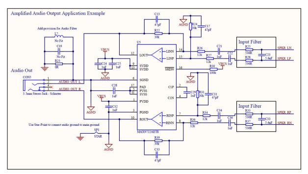
Some amplifiers do not support "capless" operation and require ac coupling on the input and output of the amplifier. Series capacitance can introduce clicks and pops during turn off and turn on as voltage transients occur across the capacitors causing audible spikes on the audio output.
